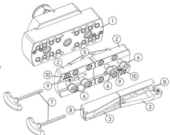
The table determines the components such as extension slide ①, clamp bases ② and insert holders ③ for each diameter range and shows in which position the clamp bases ② have to be mounted on the extension slide ①.
